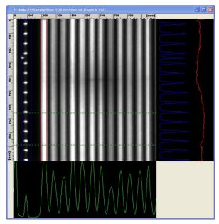
Image display includes display of rulers, multiple regions of interest (ROIs) with optional display of profiles inside or outside the image area. The look up table (LUT) is used to adapt the dynamic range of the image data for display and allows visualizing even very faint images clearly. Black and white or pseudo colors can be used for display. In very critical cases a nonlinear LUT can be applied to visualize the image. For special cases like
