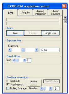
The HiPic software allows controlling and utilizing all camera features such as binning and sub array mode to adapt the camera to the individual measurement conditions.
